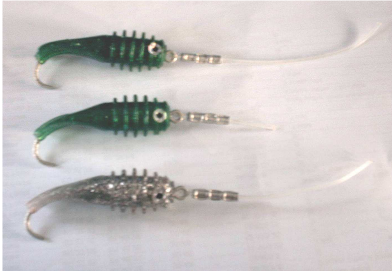
Figure 8 Sonar lures with point of hook broken off. NB Sonar lures were supplied by SonarLure.com. Lure rigs were constructed using a similar pattern to that used for making Red Gill rigs.
