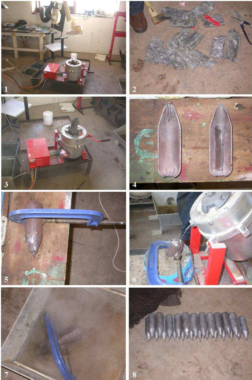
Figure 4 Procedure for producing lead sinkers; 1. apparatus used in the construction of sinkers; 2. lead is broken up into small pieces; 3. lead is placed into melting pot until almost full; 4. an eye with a swivel is placed into the mould; 5. mould is fastened using a G-clamp; 6. lead is carefully poured into bottom of mould; 7. mould is cooled in water; 8. finished sinkers.
