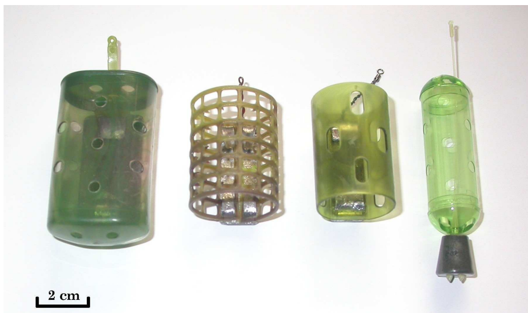
Figure 62 Perforated swimfeeders trialled for potential use as a method of delivery of pheromone pastes.
